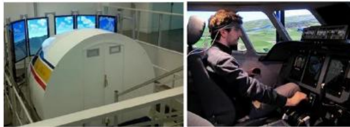
Figure 1: The PEGASE flight simulator, halfway between high-end simulation and individual computer simulation, is ideal for human factors and cockpit assistant research.
