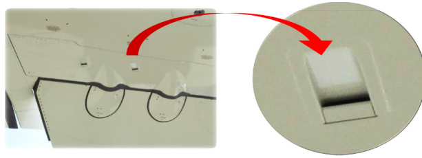
Figure 5.8: Air intake under the wing to cool the aileron actuators on an Airbus A350 according to Maré 86 .
