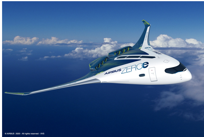
Figure 5.9: View of the blended-wing body design by Airbus in its programme ZEROe
