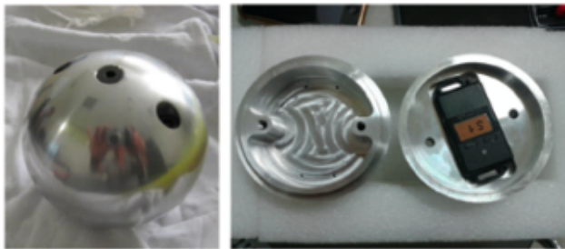
Figure 2 : The dynamic penetrator that will be used in the laboratory experiments (e.g., Murdoch et al., 2017, 2021).
