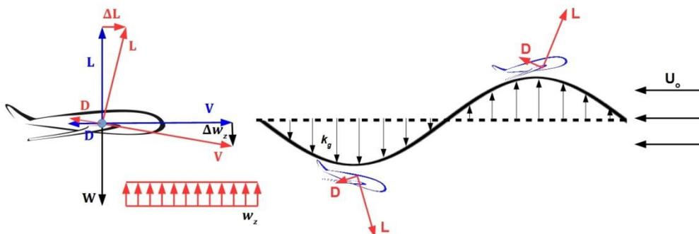
Figure 1 Gust energy extraction mechanism
