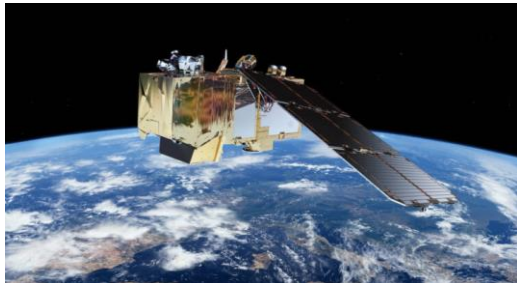
Sentinel-2 satellites carry a single multi-spectral instrument (MSI) with 13 spectral channels in the visible/near infrared (VNIR) and short wave infrared spectral range (SWIR)
