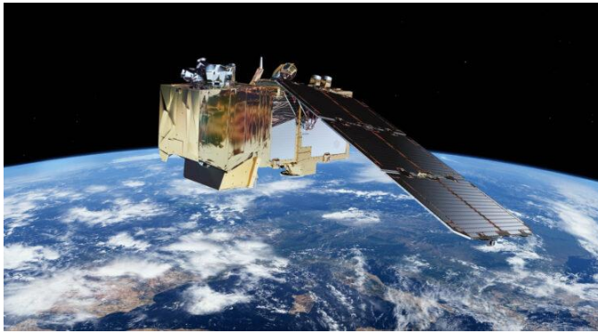
IASI-NG (Infrared Atmospheric Sounding Interferometer- Next Generation) instrument embedded in Metop-SG satellite
