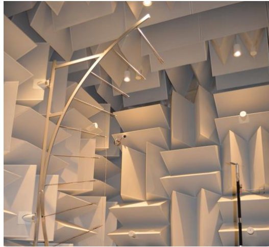
Figure 1: Experimental setup in the anechoic room for the study of rotor noise at ISAE-SUPAERO
