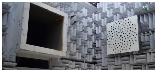
Figure 1: Microphone array measurements in ISAE-SUPAERO aeroacoustic wind tunnel.
