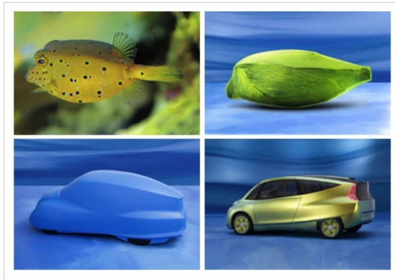
Figure 1: Computer-generated model of a Mercedes-Benz with design elements inspired by the hydrodynamically efficient boxfish.
