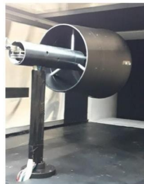
Figure 5: PropHyDis, experimental ducted propeller in the SaBRE wind tunnel
