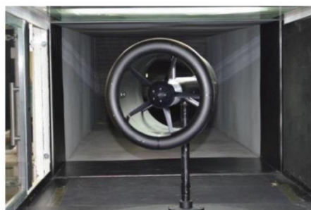
Figure 5: PropHyDis, experimental ducted propeller in the SaBRE wind tunnel
